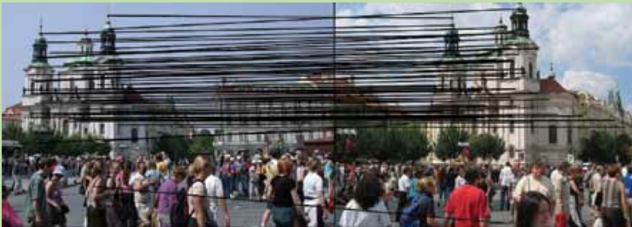
(c) a pair of overlapping images shown side-by-side with matching features connected by black lines
