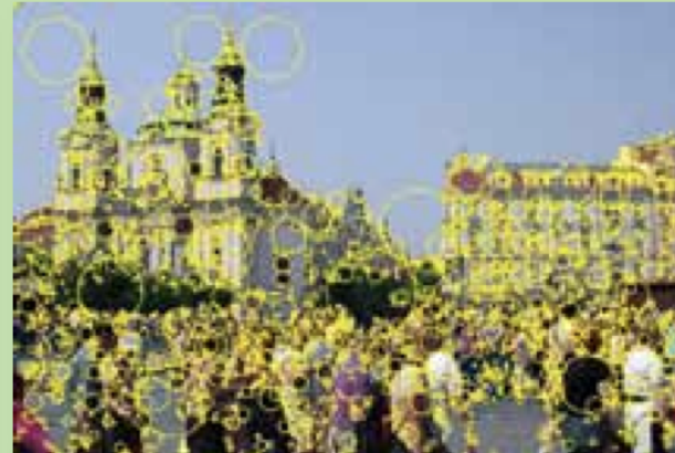
(b) input photo with extracted SIFT features superimposed
